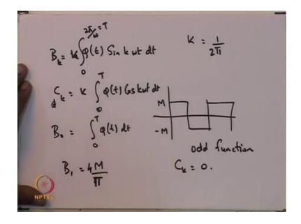
So, the Fourier series for the square wave if found by for example, b K, the way you would find b k is multiply phi t to sin k omega t. Then, take the integral over a period, so here of course omega t i sin case of t if you are taking the period in case of t you could take this integral from 0 to pi by omega that is capital t, which is the same as capital t. Then, this there would also be a multiplication factor in the multiplication factor, let me let me just call it k capital K.
