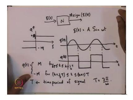
So, we are looking at the Nonlinearity, one linearity and the nonlinearity does the following if the input is psi t the output is the sin of psi t, the best way to draw this nonlinearity, the characteristics of this nonlinearity the input is psi. The output when psi is positive, it gives plus 1 and when psi is negative it gives minus 1.
