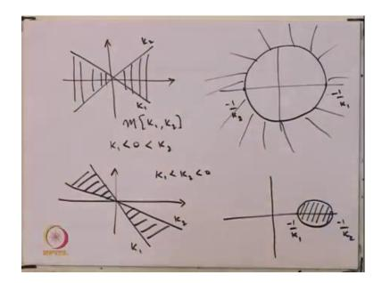
Now, further if you have a non-linearity. So, let me draw the axis and you have a non-linearity which lies in this area. So, that non-linearity is in the k 1 k 2 sector. So, this is k 1 this is k 2, where k 1 is less than 0 is less then k 2. Then what the circle is criterion really tells us is because this is less the k 1 is negative. Therefore, minus 1 by k 1 is up here and here somewhere is minus 1 by k 2.
