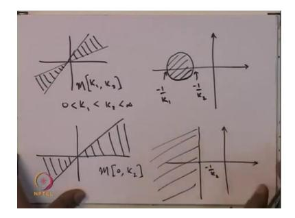
So, the non-linearity is in this shaded region. So, the non-linearity is between k 1 k 2 where k 1 is positive less than k 2 less than infinity. What this translates to is a circle, this is the point minus 1 by k 2, this is the point minus 1 by k 1. The forbidden region is the shaded part. This is what we first showed. Now, if the non-linearity is expanded such that the non-linearity is in this sector like this. So, the non-linearity now is in the 0 k 2 sector then what this translates to here.
