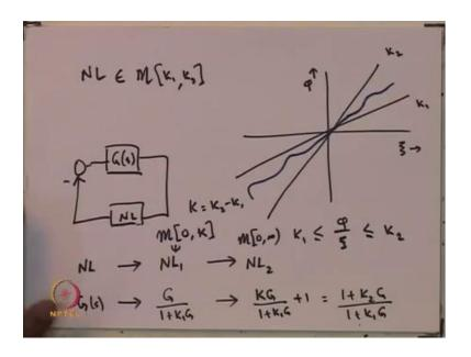
So, suppose we consider a non-linearity, which is in the k 1 k 2 sector. So, what we mean by that is if you think of psi as the input to the non-linearity and phi as the output to the non-linearity. Well there is this line with slope k 1 and there is this other line with slope k 2. What we saying is that the non-linearity is such that it lies in the k 1, k 2 sector. Of course, the other way to talk about this is that phi by psi is, this thing is greater than k 1 and it is less than k 2.
