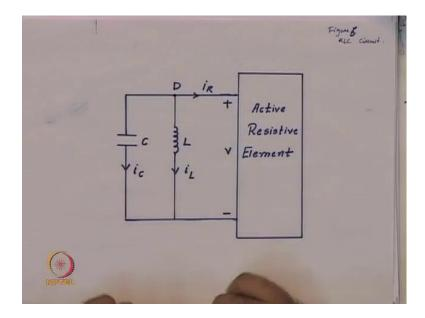
Now, for the example of the van-der-pol oscillation we will consider a RLC circuit, where R is the active resistive element. Now, let us consider this figure in this figure this is an RLC parallel circuit this is a capacitance c which is greater than 0 L inductance which is greater than 0 and we have connected in parallel active resistance element, this we is having v i characteristic as i equal to capital H of v, where we had defined capital H of v before.
