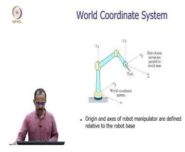
So, I already mentioned this world coordinate system, the basic coordinate system is known as the world coordinate system and this is known as that tool coordinate system. So, origin and axis of robot manipulator are defined relative to the robot base. So, we have the robot base and then we define all the coordinates with respect to the robot base.
