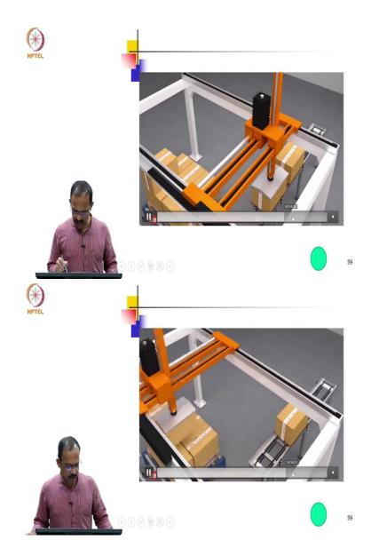
And the third one is the 3 prismatic joints, which we call it as the Cartesian robot. So, this Cartesian robots are again used for pick and place applications. The only difficulty with this kind of robot is there the space required for them is large compared to their workspace otherwise, they are very easy to control because all the three motions in x, y, z axis so it will be easy to control. So that is the advantage of having this robot.
