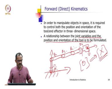
Now, coming to the forward kinematics relationship, so as I told you, you have a robot so you have 1 joint here, and then you have another joint, a joint here. It can be a rotary or prismatic
