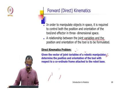
So, we can define the direct kinematics problem as given the vector of joint variables so it can be theta or D prismatic joint or rotary joint so generally we define it as a joint variable of a robot manipulator determined the position and orientation of the tool with respect to a coordinate frame attached to the robot base is known as the direct kinematics problem or the forward kinematics of the manipulator.
