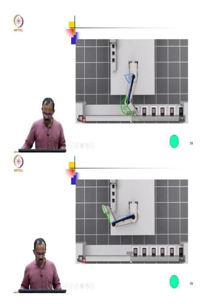
So, you have the last 1 is the prismatic joint and then 2 rotary joints and all the joint axis are in vertical direction. So, this can be used for positioning and assembly applications and it actually provides you a compliance in the horizontal plane because all the joints are in the vertical axis and the workspace of this is shown there.
