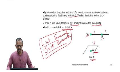
Now, we will look at this and then define how these parameters can actually be defined in the case of a manipulator. So, first we start with the links and joints, so we will start with the link zero and then joint 1, then link 1, joint 2, link 2, joint 3 and link 3. So, this is the way how the links and joints will be numbered.
