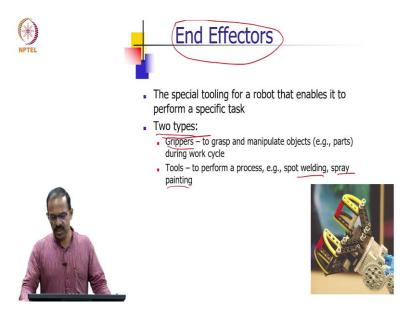
So, we discussed about the body and arm configuration, we discussed briefly about the wrist assembly and the wrist actually can have different ways of assembling these joints, it can have a spherical wrist also, where all the 3 joint axis intersect, we will get a spherical wrist. And at the end of the wrist you will be connecting the end effectors, the end effectors are the tools which are attached to the wrist assembly in order to get the necessary work done.
