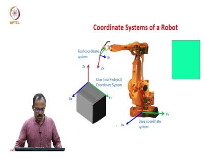
So, most of the time what we will be doing, we are interested to know the position of the tooltip, and if you move these joints how these tooltip gets affected is the relationship we are interested in, that is where we want to know the kinematics. So, if we supply these joint values theta I put just these joints parameters as theta, if I substitute these values of the theta, can I get the position x, y, z of the tool is my problem.
