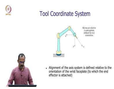
And that tool coordinate system, so we define this as the tool and then we define a tool coordinate system, and we define these coordinates based on some criteria. So I will explain that how do we assign the coordinate frame later, but we will be having 1 coordinate system at the tooltip.
