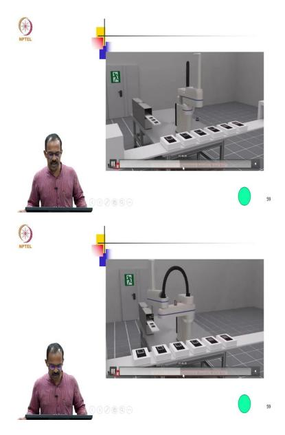
Now, it's the second one is the SCARA configuration, you can see that there are 2 R joints and the 1 P joint.
