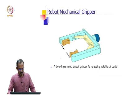
So this is a example for 2 finger mechanism for gripper. So normally gripper is not continuous part of the robots, and therefore the motion or this degree of freedom is not added to the robots degrees of freedom. So we will be having six degrees of freedom for the robot, but then the gripper will be having additional degrees of freedom.
