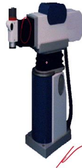
Example of a Cylindrical Work Space Robot
