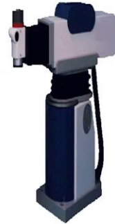
Example of a Cylindrical Work Space Robot
