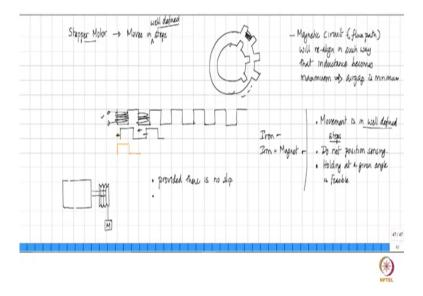
So, one other electric motor that is used in such cases is is known as the stepper motor. The main advantage of this is that it moves in steps and that is an advantage as well as it is a disadvantage. It moves in steps, but it moves in well defined steps. So, that is the major advantage of this machine. So, essentially if you are going to have a machine that has a stator and the rotor, so the stator then has slots like that and so on and the rotor has extensions like this.
