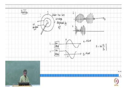
So, one can go a little bit more into this and have another entity known as resolver. In this case, this is again an electromagnetic equipment you have a stator and you have a rotor, coils are there on the rotor, I will just show it as two leads and you give a high frequency excitation to this. Stator has two windings displaced by 120 degrees, displaced by 90 degrees and the rotor is then linked to your system, electric motors for which you want to determine the rotor angle.
