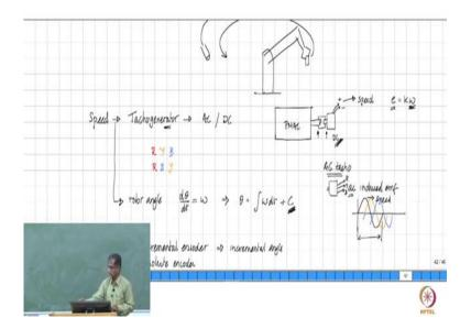
But on the other hand, if you are going to use electromagnetic equipment, which is like what we saw here, especially if it is in AC Taco. Here, you do not have a difficulty because you are only looking at induced EMF and dust is not an issue at all.
