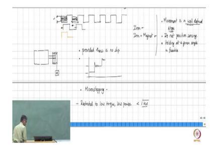
Then if you want the rotor to move by a step, what you are actually saying is that you are going to energize something on the stator and the rotor will then snap into the next location. And when the rotor is going to snap into that location, no mechanical system is an ideal mechanical system. Imagine if you want something will snap into location it means that that must have a high acceleration and the velocity must then go to 0 exactly at that position, which is impossible.
