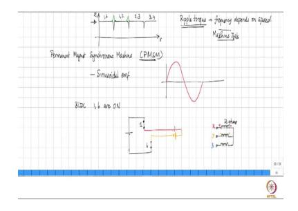
So, the machine looks very much similar to this in the sense that the field arrangement is put on the rotor, the armature placed on the stator. No change in that, but the induced emf in the first case was a flat top emf; whereas in this case the induced emf will be sinusoidal. You will have a sinusoidal emf, so you are going to have a sine wave that is vary respect to time; now, this bring about more difficulty in operating the machine.
