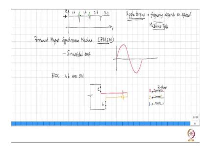
At this instance or around that interval around that instance; what you will have is if you plot the electromagnetic torque versus time let us say. And during this region device is 1 and 6 were on, and then it has to go to 1, 2. It will not go smoothly like this, what will happen is invariably there is likely to be a dip. Similarly, after device number 1, 2 finished, you go to device number 2, 3;
