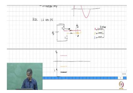
And therefore, what will happen is in the first 60 degree interval; when you are having the voltage of the R-phase is high and the voltage of the Y-phase is low. This is emf plot if I draw the flow of current I, then during this interval the current is also flat; current meaning this current that is going in. So, the fact that flow of current is steady ideally is ensured by the fact that the circuit is a DC circuit.
