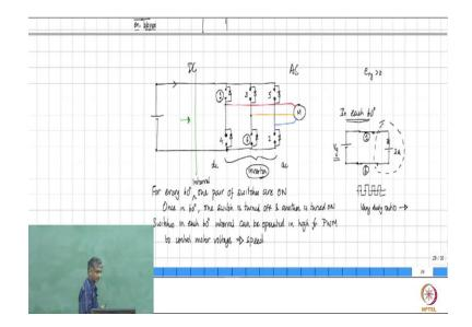
And therefore, you make use of a circuit as we had discussed in the last class that is here. And this is then called as an inverter that accepts DC on the input side, and delivers an alternating AC AC output voltage, which is then the given to the motor. The understanding of how this is supposed to operate was what we discussed in last class.
