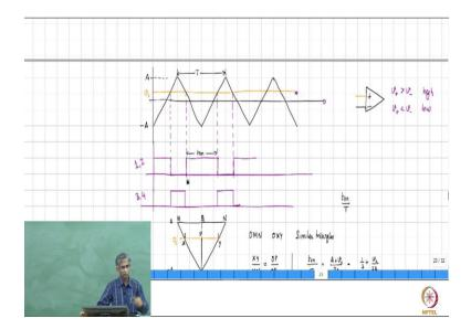
So, this we implemented by means of having a high frequency ramp signal; and comparing it with the output of the controller to generate this kind of a waveform, switching waveform. So, here also we do the same thing.
