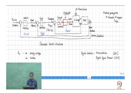
But, when it comes to the final stage that is here, this block which we said is going to is going to take the output of this controller. And then convert it to switching control signals.
