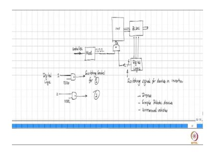
So, what we will do now is then you have the BLDC motors here, and BLDC motor is connected to the inverter. And then you have the shaft and then you have Hall sen... switches that are placed here. You take the output from the Hall switches, and then you have a digital logic that is placed here. This digital logic in turned gives you six signals; each of which determines when a particular device is going to be on or off.
