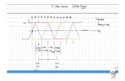
So, these machines are best design as 3-phase machines that means all the different conductors that are put around the circumference of the stator are split into groups, 3 groups, each group is than called as one phase. And therefore, we then talk of induced EMF in each phase. So, one of the ways in which that can be done is like this, the induced EMF can be made to look like this. So, this is a trapezoidal EMF and not a sinusoidal induced EMF.
