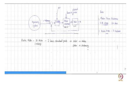
So, you may represent it in this manner that you have the motor and then you have the power electronics and this gets in source of power one may call it tools of electrical power. This is what energizes an electric motor and then you have a shaft which may be coupled to whatever application we want. This now needs to be given an input so you need to have something here, which say how this electronic circuit should act in order that the output performance is achieved.
