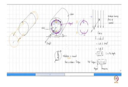
So, this member the outer member which is called as I said stator is fixed in some way to a base you may put a bolt and fix it. And therefore the stator is stopped from rotating and this member which is inside, this is then called as the rotor, the rotor is free to rotate. And your application whatever you are going to connect is then connected to a shaft which extends from the rotor. It may not be as long as I have drawn, but there is a shaft which extends from the rotor.
