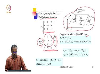
So, we know this subject grasping by the robot, so the tool gripper orientation is given like this and therefore the tool to base will be like this. So, now the position of the object is this but the gripper is in this orientation, so therefore the tool to base transformation is given by this 1 minus 1 minus 1 30, 15, 1. So, this is the tool to base.
