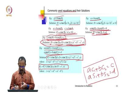
So, we will they see what are the standard form that we can use, or what are the commonly used equations in this kind of equations and then how do we solve it. So for example, if you have a is equal to b sin theta as a form, if a is equal to b sin theta then we can write sin theta is equal to a by b and cos theta is square root of 1 minus a by b square and therefore, theta can be written as atan 2 a by b square root of 1 minus a by b square.
