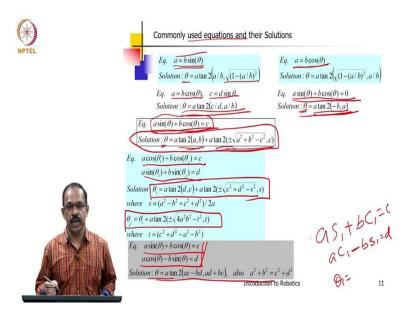
Another one is, this is a sin theta plus b cos theta is equal to c, a sin theta plus b cos theta is equal to c, a cos theta minus b sin theta is equal to t, that is the relationship, then solution is this one, ac minus bd ad plus bc a and c are known b and d are known therefore you can directly get this as theta is equal to this. So, this is again format of a s1 plus b c1 equal to c and ac 1 plus, ac 1 minus minus b s1 is equal to d that is the format here.
