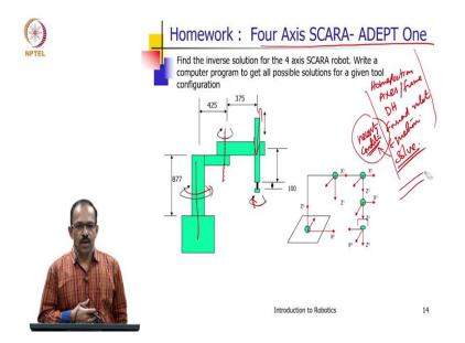
So, this is an home work for you, so you can consider a 4 axis SCARA robot, it is ADEPT one SCARA it is a commercial industrial robot and we need to solve for its inverse problem.
