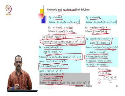
So, in the previous example actually we solved it and then got the same result what we are seeing here like PX is 11 c1 plus 12 c12 and PY is 11 s1 plus 12 s12 it is the same format that you can see. So, 11 c1 plus 12 c12 11 s1 plus 12 s12 and then we saw that c2 is PX square plus PY square minus 11 square plus 12 square by 2 11 12 which is the same as this and the same way we actually solved it for solved for s2 also by substitution.
