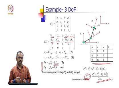
Hello, welcome back. So, we are discussing the Inverse Kinematics of Manipulators, in the last class we briefly mentioned about the method by which we can solve the inverse kinematics and we took a very simple example of a 2 degree of freedom planar manipulator to show how the equations can be solved and then we consider a 3 degree of freedom manipulator a planar manipulator as shown in the slides.
