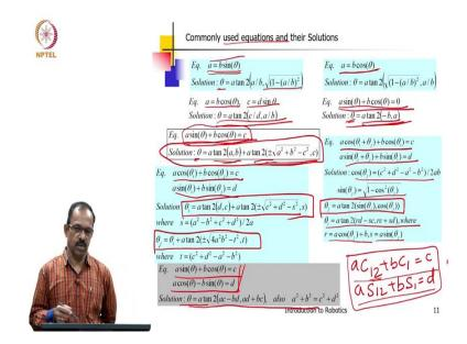
The next one is another format a cos theta i plus j theta i plus theta j plus b cos theta i is equal to c a sin theta i plus theta j plus sin theta is equal to d, that is you have a cos theta 1 plus theta 2 plus b cos theta 1, so it is a cos I will write it as 12 a cos 12 plus b cos 1 equal to c similarly, a sin 12 plus b sin 1 equal to d.
