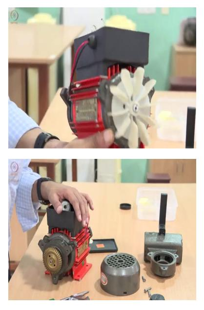
If you look at it, this does not have what is known as a volume case so, you can see the casing more or less it is uniform throughout in case of a volute casing you will have a gradually expanding outlet please take a look at the construction of a standard centrifugal pump it is called as a volute casing; v o l u t e, volute casing.
