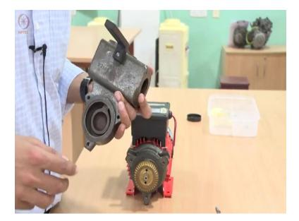
So, this is especially impeller so, these impellers you will only find in self-priming pumps. So water enters this way so, it basically enters tangentially here so, impellers carries the water remember this entire top portion and the casing is filled with water and then it goes around and then, exits and then comes out to through the top.
