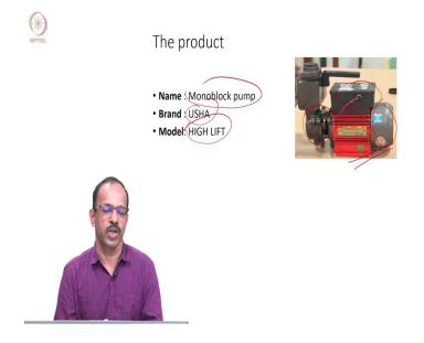
So, the Monoblock pump we are using is shown here so, this is again, an USHA make and it is a high lift model so that is the pump you can see. So you can see there is an electric part you can see there is an electric supply and then there is a motor and there is a pump body and then you have this assembly over here which will take input and then deliver the output.
