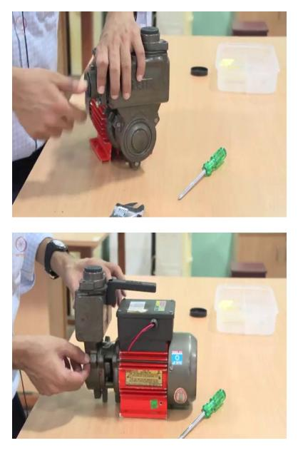
To summarize what we have learned today, basically, we have learnt about a self-priming mono-block pump that is capable of priming itself. In case of a normal centrifugal pump, a pump that is called a non-positive displacement pump, what is a non-positive displacement pump? The pressure is dependent on flow in case of a positive displacement pump pressure is independent of flow.
