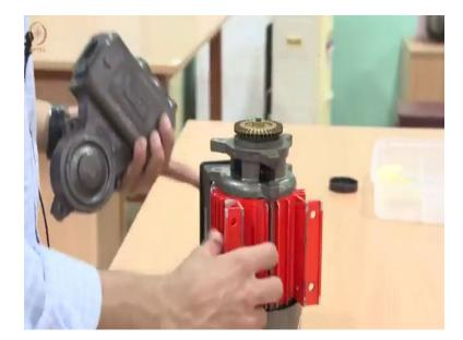
But today, we are going to look at a special type of a pump so, this is a pump where in you do not have to basically fill the entire suction line with water it is only enough that you fill this portion just by removing this so, you just have to fill in only this casing, just maybe half a litre of water you pour in so, you have a separate provision for that you open this you put a funnel and then you fill it with water, only this portion.
