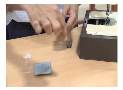
So you take a single piece of thread and then you keep looping it around with what we call as a bevelled needle. So we do that. That is called as a chain stitch. So that is one of the earliest forms of stitching.
