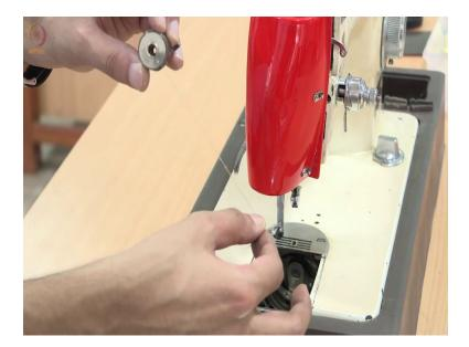
Now, how do we regulate tension at the bottom part of the spool? So remember, we basically spool this bobbin using this mechanism. Once it is spooled, we put it inside this housing here. Again, we have a tension regulatory mechanism. So if I simply put it, if I pull it, you can see there is no resistance, it is simply rolling off.
