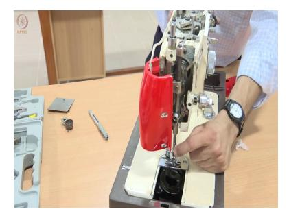
So basically what we will do is during threading, so it is called threading the machinery. So it is quite an elaborate procedure. If you have a sewing machine at home, I encourage you to please explore it on your own. So you thread it like this.
