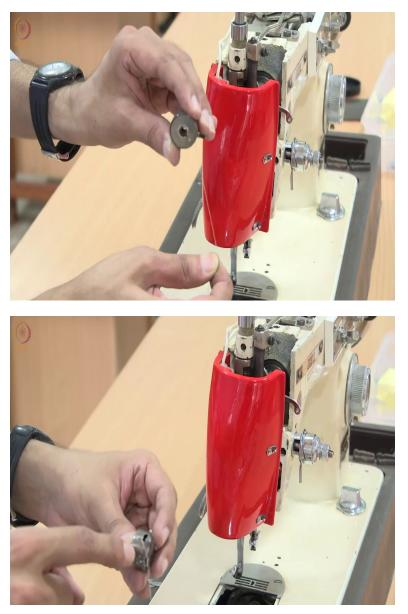
So how do we regulate tension? We have another spring here, a pre-loaded spring. So how you load it, I hope it is visible on the camera. So you take a certain free portion of the thread and then you pass it underneath this spring.
