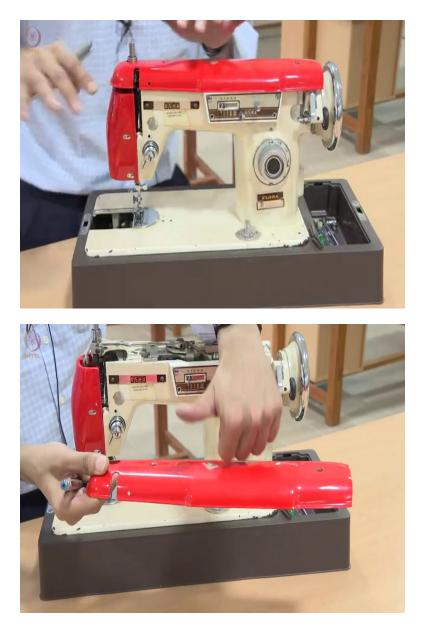
Let me start by dismantling the top cover. So let us first understand the machinery, overall machinery. So let us understand the overall machinery. So this is a very old model. You can see it is made of cast iron. It is pretty heavy, this machine weighs something like 10 kilograms, and it is pretty heavy to move around.
