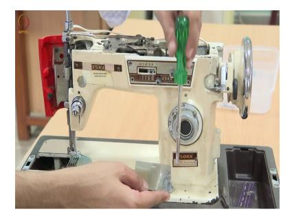
Now, in addition to that, if the needle had only travel up and down, it will be doing a linear stitch. Just think about relative motion, so it is just doing this. Now, as it is advancing, I am also giving a lateral motion to the needle. In addition to the up and down motion of the needle, there is also a superimposed lateral motion.
