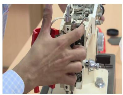
So far what we have seen is we have looked at the crank slider, we have looked at another crank slider that moves the needle up and down. We have another crank that basically drives this lever.
