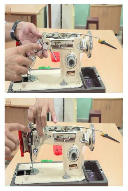
Keep in mind that these are special screws. This screw also functions as a bearing. You can see this is what we call as a shoulder screw. So it does not have to thread all the way through, there is a smooth part of the screw, and then you have the threaded part. This function is what is called as a bush bearing.
