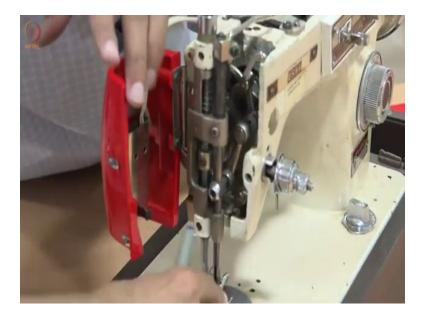
Now let us go one by one. We have what is called as a crankshaft. This is called as a crankshaft. You can see this is a common shaft and this is called as a crankshaft. If you look at any internal combustion engine, it has a four-bar mechanism; it has what is called as a crank slider. In this case, it is flipped.
