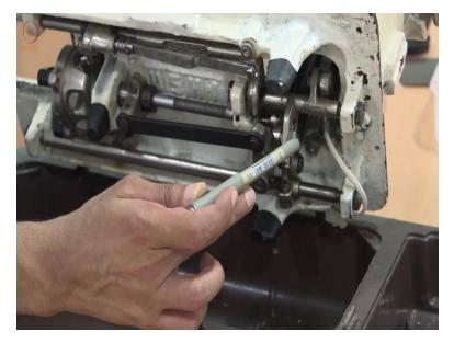
You have a slotted lever, so this mechanism is called a slotted lever mechanism. So you can see, so basically we have turned a rotary motion. Using a crank, we have turned it into an oscillatory motion that drives basically another slotted lever. And there is a sliding block that is connected to another crank that gives you an oscillatory motion.
