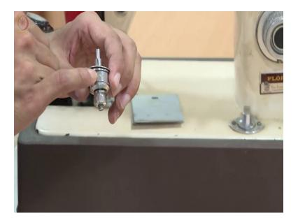
The reason why we have this is, so there will be spring here. So basically, when I tighten this, it puts, what is called as a clamping. So you can see here as a thread gets wedged between these two plates here. So this is how it is wedged. As the thread gets wedged, when I tighten this, it puts... it increases the clamping force, which means it will basically increase the tension on the thread.
