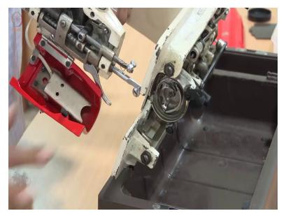
This goes inside like this. We remove this lever, one is broken. Now, in this construction, some machines will have it in this way, some machine, Singer, will have this entire bobbin facing this way, that is, 90 degrees; this entire mechanism will be rotated 90 degrees. So that depends on the manufacturer.
