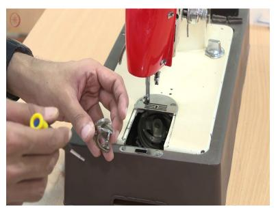
What happens is when this creates a loop, you can see it is quite sharp. And then you can see there is a slot here. So needle goes through this. So I will show you the, how to spool this spindle here. This basically takes the thread, it comes like this. So when it goes through this that entangles the thread.
