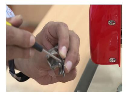
Once you put the spool, once you thread it in place. So this will be like this inside. And then all you have to do is put it and then press it. Now, this locks in place. How do you remove this? Basically how to pull this lever and then take this out.
