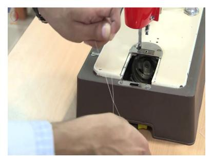
The reason why you have such complicated machinery is you have to basically, so this is the bottom part of the mechanism that basically synchronizes the movement. For instance, imagine this is the needle. So a needle is connected here to this lever. So when the mechanism goes up and down, it goes up sorry, when the mechanism rotates, it goes up and down.
