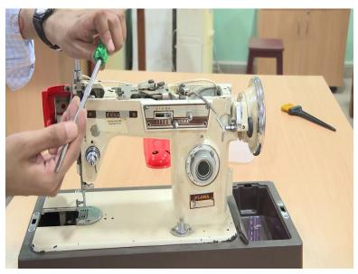
If you observe in a screwdriver, we have these flats here. So when you engage a screwdriver, so this is a multipurpose screwdriver. I have a flat bit here and I have a Phillips head here, depending on which one I want to use when I engage it, I just cannot put it like this because I am not constraining the rotary motion since I am applying a torque.
