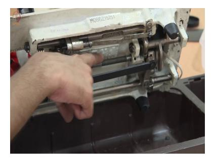
You can see this shaft, this bottom part basically oscillates. How does that get that oscillatory motion? So this is connected to a shaft here. And where does that shaft connects? It is connected to another crankshaft here. It is connected to another crankshaft here. So this shaft, it is connected to another crank.
