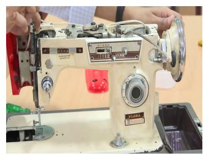
Now imagine me manually moving this. So this is what I spoke about, synchronizing different motions. So you have what is called as a positive linkage. You cannot have a belt drive here. Belt drives typically are used, I mean, you will find them in sewing machines.
