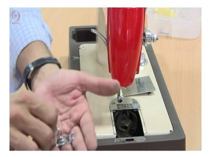
When you feed a cloth, this is how you will feed a cloth. So this is how you will feed a cloth. This puts a pressure so you have another lever here that moves this shoe basically that rests on top of the cloth and put some pressure. So this is another mechanism. If you look at it, I do not know if it is clearly visible on camera.
