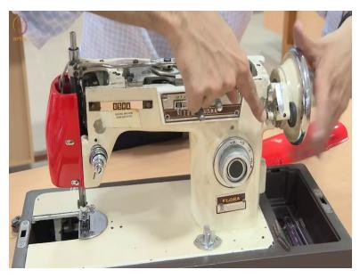
Imagine, on top, I have another thread supply; I have an external threaded bobbin. So I take it and then I feed it here. So what happens this starts once a power the machine. So basically, you can see it is rotating the spool, and it will start winding this spool.
