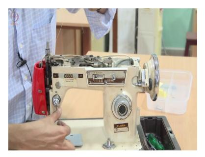
And the tension can be regulated by the screw here. So when I spool the, when I first thread it, I will put it through this and through the lever. So the thread will, so let me just show you quickly.
