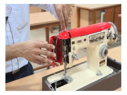
Typically, if you look at a modern sewing machine, so this is, even though I call it modern, this is actually, this machine is about 25, 30 years old. So this machine uses what is called a lock stitch.
