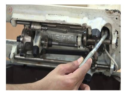
So that connecting rod that you saw. It is this connecting rod. So this connects here. So this connecting rod here; so this connecting rod here, so this is the connecting rod that I am pointing out. So this is the connecting rod I am pointing out, this is the bottom part of it.
