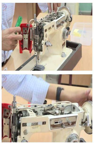
How does this motion come? You can see there is another lever mechanism here. So when I engage it, you can see at the top this lever that you see here basically gives you the oscillatory motion.
