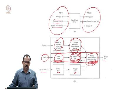
For example, if you look at the nailer, you can see these are the input energy, material and signal. So, the energy is electrical energy if electrically operated plus the manual energy will be there. And then you have this material that is the nails going inside and then the signal is further tripping or dispatching that or that kind of information that you are getting. So, you
