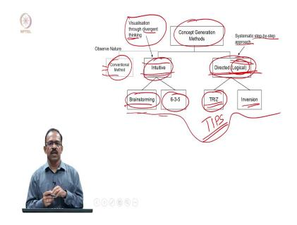
The concept generation methods can be classified into mainly 3 categories. So, one is the conventional method, the other one is known as an intuitive method, the third one is known as a directed or logical method. The conventional method is the one which actually we normally follow without really going through a very structured method, we will look at nature and then see what are the ways in which the natural source is a particular problem.
