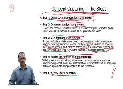
This is what actually you are doing during the lab exercises also. We are actually asking you to open a product and then try to identify the components and map the components to the functions and then to get a particular function what concept is used by the designer. So, by going through multiple products, you will know that for the same function you can have
