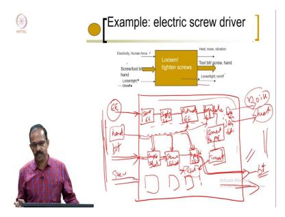
Okay, so we will get this as loosen or tighten screws. So, electricity and human force as the inputs. And then screw the tool bit and hand, okay hand also as a material will be going inside. And then loose or tight, or on or off will be the information. And we will be getting the tool bit screw and hand heat, noise, vibration and loose or tight, or on or off as the material.
