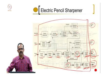
The last example for today is the electric pencil sharpener. As you can see here, electricity is going inside, the hand is there and the pencil is there. And you get the vibration as an output, noise as an output and then the sharp pencil as an output and some gravity forces will be there and the shavings of the pencil will be coming as an output. Now what is happening to electricity?
