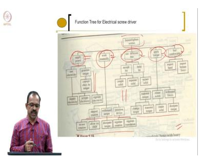
Once we identify this function, we will be able to create a function tree. A function tree is one, you will be having a top level function at the top and then we will try to identify the main functions needed in order to get the top level function. And then we go for the all sub-level functions at the bottom level and then create a tree structure with all the lower level functions
