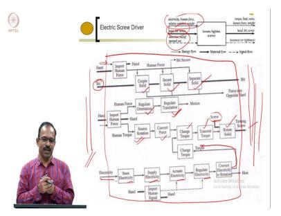
Then I will take this as a more detailed one, I would like to show you the detailed explanation. So this is the inputs, as I showed you the input going and then output. As I told you the tool bit is coming and then coupled solid, secure solid and separate solids, okay? We will be using the hands, using hand and human force to do this so we need to have the hand and human force to do the solid, coupled solid, secure solid and separate solid.
