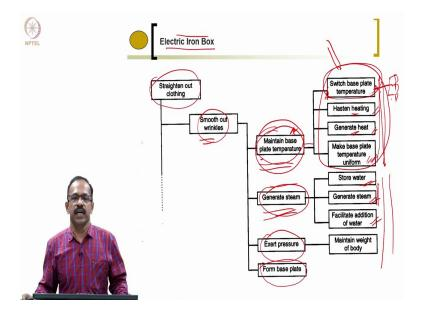
Just to give you one more example about the functional decomposition or the function tree, so this is an iron box, electric iron box. So we can see that in an electric iron box, the top level function can be assumed to straighten out clothing. So that can be considered as the top level function and you can have additional things also. And then, smooth out wrinkles will be the way how you can straighten out the clothing.
