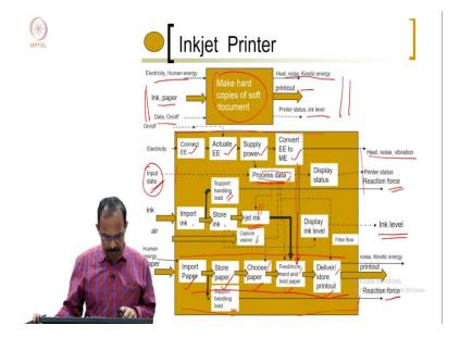
Okay? So this another example for the inkjet printer. So we are talking about the printer, and in the printer, we will see that the main function is to make hard copies or soft copies of the product, of document and the inputs are the electrical, electricity, human energy, ink and paper. And here you have this heat, noise, kinetic energy, print out, printer status and ink level. So these are the inputs flows and these are the outputs.
