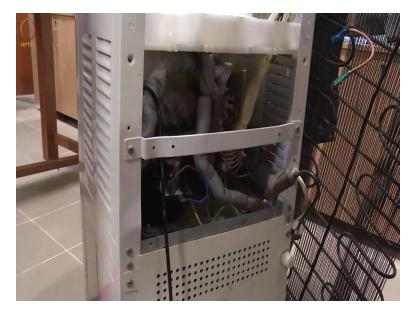
So, for example, this is one component of how the copper tube is connected to that component, then from that component where the copper tubes are going. So, just draw a diagram if you can. So, the first compressor, this part is the compressor, this black part.
