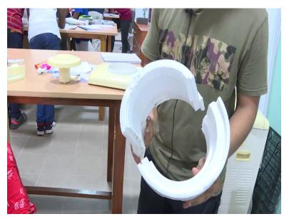
These are thermocol pieces used to insulate the cold-water chamber.
