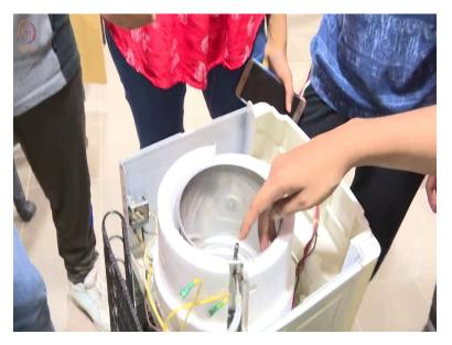
Student1: Exactly, so basically the cold water is stored here, in this particular chamber and this thing insulates it, so just remove the thermocol. Okay, anyone heard of a term known as thermostats? You know what they are?
