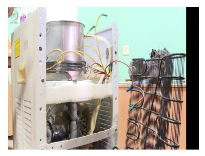
Student1: Yes, this full black part is the condenser, so this is the evaporator. Now, see this thin tube it goes here, it winds here. Then, yes, this is our cooling chamber, then it goes here down, this is the tube, it goes inside so our refrigerator is our second cooling chamber, from the refrigerator it comes back to the compressor, so this is the cycle. So, this is how the cooling is done.
