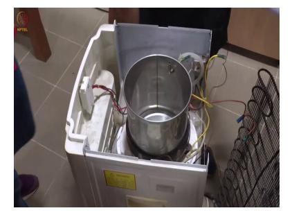
So, this is like latent heat, this is something like latent heat. So, what happens is, this gas starts evaporating from a liquid state, now it needs some heat to evaporate, okay? So, these tubes are wound about some chambers, so in our particular case this is that chamber and in case of refrigerator, refrigerators are also that chamber and the heat that the gas needs to evaporate it takes from the chamber. So, now imagine if water is kept here and this gas is extracting heat, what will happen?
