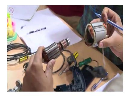
Field magnetic and the connection of armature magnet are both connected in parallel and in case they are connected in series it will be series DC mall and the thing is, so right now I have, so you can see that essentially if I take a quarter of this coil I have 1, 2, 3, 4 so there will be 16 such armature coils passing around you. So essentially how can you visualize it?
