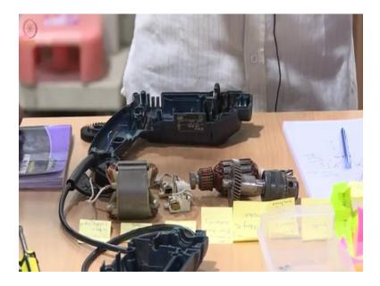
The other thing is, when you saw that the motor was fixed here, I was trying to move this, but I was not able to move it. So there must be some sort of interlocking structure that was preventing it from moving. Have you noticed it? When I removed the outer casing, I thought I was trying to move but it was not moving.
