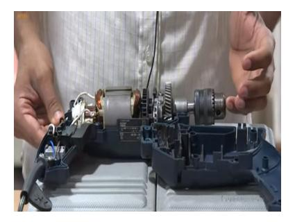
The second one is gears. So where are the gears? So these are the gears. We have found some sort of a gear and the third is a drill bit. So drill bit is some accessory that will be provided and all. On-off switch. We have an on-off switch, but what are the components that we are not able to guess? We noted that there are some vents on the product.
