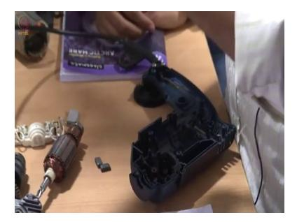
This is the ball bearing. This is the entire drill bit. So I will rotate this. The ball bearing will roll but it will not allow any motion in the axial direction. Is this clear? So this is essentially a mode switch and I told you the mode switch was essentially used for drilling motion. In the case of drilling motion which will come into play the spring or the ball bearing.
