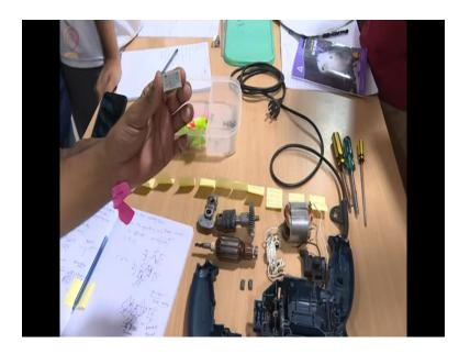
So a capacitor can have essentially 2 functions. It can be used for the working of the universal motor as well and the second thing is for, it can store some sort of energy to prevent the jerky motion or to avoid back EMF. So we saw that, so what does back EMF mean? The thing is, I am moving so essentially told that this is a current carrying coil.
