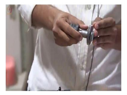
This is the interlocking machine. So try to rotate it in this direction. Try to rotate in a clockwise direction. No-no hold this. You will not be able to move. The thing is if this joint is tight enough right now what is happening is, I am not able to hold it. This joint is tight enough so it will have rotation in one direction is possible but rotation in the other direction is not possible.
