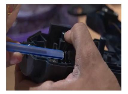
And in case I am drilling steel or any other structure where I need the drill bit to be entirely rigid. I do not need it to move. So I will have a ball bearing in this direction so that it will not allow any motion but I need to support the rotary motion. So ball bearing will essentially slide in this place.
