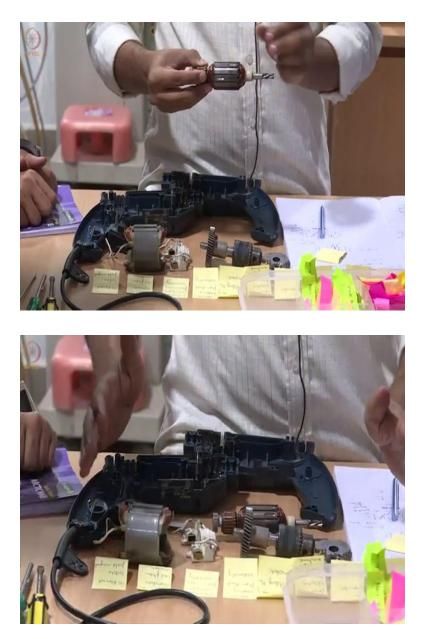
So this is the commutator. This is the armature coil and this is the field magnet. So due to the magnetic field interaction between the field magnet and the armature coil it leads to rotation of a motor and this is what kind of motor. This is universal and it is up to you to find out how this works. I have given you a hint. A rectifier circuit will be used.
