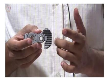
You have seen this in engines. So the thing is I want to dissipate heat, I need to have some sort of a surface area which is so these are essentially called our fins and where can you see this? The corners of the engine will not be smooth. It will have some sort of a corrugated surface. So more the surface area is the amount of heat dissipated in it.
