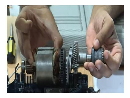
Yes, so I am able to remove the entire casing. So, first I will remove this enter chuck assembly.
