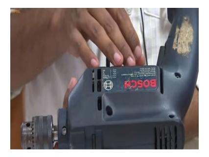
It is given that it is operating at 220V. 220 Hz, so that is, it is operating on AC and the second thing is given is the RPM. So the drill bit that is provided with this you can see here. It's written at 8  $\phi$ . When you notice  $\phi$  on any of the machining components it is essentially the diameter. an 8 mm drill bit is provided with this drilling machine and apart from that you can notice that it is 2800 RPM(min<sup>-1</sup>).
