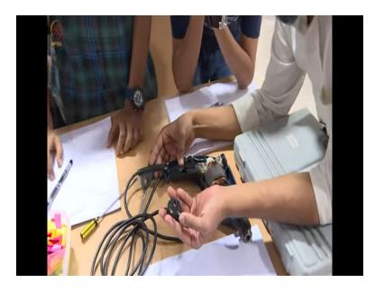
These 2 are the power cords that are going to the machine. So I have a capacitor here which will charge and discharge and it will just avoid it from having the jerky motion. So in case it will have some back EMF, it will be able to control that. So what is back EMF and how is the interaction happening inside the motor? I will explain to you when we will open the entire model.
