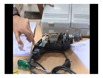
We will remove these 2, these 3 screws. You can note the third step. Remove these small screws. I have provided an AC so I have 2 wires.
