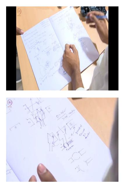
I also need to have some connections here in order to make it north and south. So the entire current that is passing from this positive and negative polarity is making this magnet a current carrying coil and also this is as a electromagnet and depending upon so I have this circuit, I have this circuit and if both of these circuits are connected in parallel, I will have some sort of a shunt DC motor. Shunt DC motor in the case of the connection of what is this?
