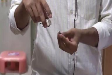
This is a 3 fingered chuck assembly and 3 fingered is used to have force closer. The summation of all the forces should be 0. We thought that it was a plastic casing but on removing that we saw that there are 2 carbon brushes attached to it by means of spring and these were spring-loaded slip rings which are in connection to the commutator.
