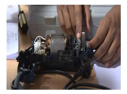
So I need to remove this too and what is this? When we remove this, we will notice what components are coming out of it and then I will explain to you what it is. Try removing this too and this is also cross headed and it is not a machine screw. So right now what I will do is, you can notice that this component takes power from the power switch and it is connected to the motor by these 2 things, these 2 wires.
