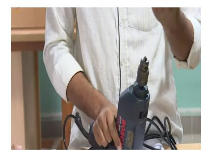
This is essentially a 3 fingered chuck. So one of the questions I want to ask is, why is it a 3 finger Chuck? Can I make it 2? It will slip. So essentially what is happening here is the contact between the drill bit and the chuck is maintained due to the force applied by the chuck. So I need to have some sort of a force closer that is the summation.
