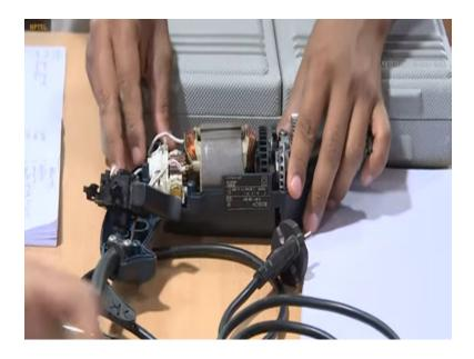
So now what I will do is, I will remove the chuck assembly from the drilling machine. So this is essentially called the chuck assembly because it is used to hold the chuck. So I will remove these 2 screws. The pitch, so you can see that here the pitch is not that uniform but in this case, it is a machine screw.
