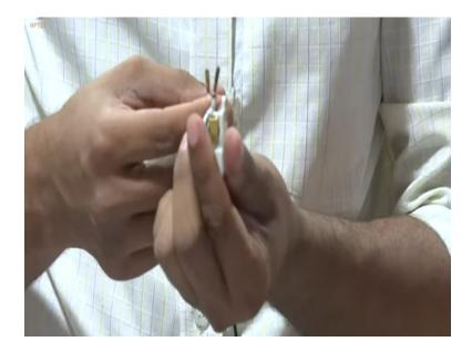
So these are spring loaded. Yes to hold it and the other thing that you can notice is due to successive rotation there is wear and tear in this carbon brush. So now I can remove this entire casing. Let me see if I am able to remove it.
