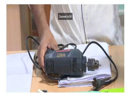
I have some source of power and essentially I will be converting into some rotational motion. So I have some electrical energy. I am converting into a mechanical form of energy. So that is what is called a machine and what is a mechanism? So essentially there are 2 kinds of things. There is something called mechanism and there is something called machine. So in a machine, we have one input form of energy and we transform that into some kind of output form of energy.
