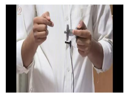
So spur will have the teeth horizontal. So in case it is helical, it will have some sort of a curve and so why is it used? If you are able to transmit a large amount of forces, we need something to have permanent contact. So line contact is better than a point contact that is intuitive, right. So we will have some sort of a helical gear between these 2 components. So this is the chuck assembly that I have removed.
