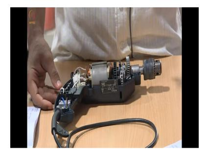
So the second component is removing the plastic casing. You can write it and paste it. Removing the screws. The second step was removing the plastic casing. So initially we noted down a few components. The one is the motor . We can find it here.
