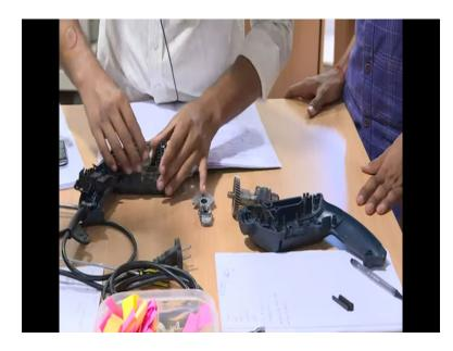
This is the component that is enclosing the motor as well as a chuck assembly. Now, what I will do is, I will remove the cooling fan.
