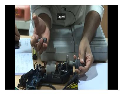
The first thing that you will notice is this is some sort of the gear and I told that gear was used for transforming motion. So what kind of gear is this? Helical bevel gear. So I will tell you
