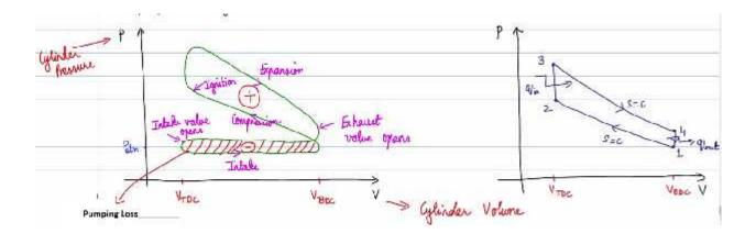
So if we look at a typical PV diagram ok of a gasoline engine right and we want to look at the various processes that happen. We typically get a curve which is in this manner, so P is the cylinder pressure of course alright and V is the cylinder volume. And naturally the volume of the cylinder varies between the clearance volume and the total volume, this is the volume at top dead center and volume at bottom dead center right.
