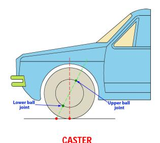
Now if we draw a line passing through these two ball joints that is what is called as the what to say from this perspective you know like it is the axis about which the wheel is going to be steered okay.
