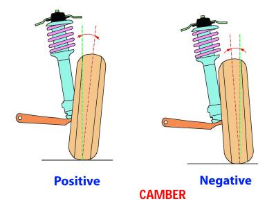
So let us say this green dashed line is the vertical axis this red dashed line indicates the central wheel plane okay. So essentially it is the angle made by the central wheel plane right with the vertical axis when we viewed from the front of the vehicle so this is what is called as wheel camber okay. So let me write down the definition it is the angle made by the wheel or tyre with the vertical direction when viewed from a front of the vehicle okay so that is what is called as camber.
