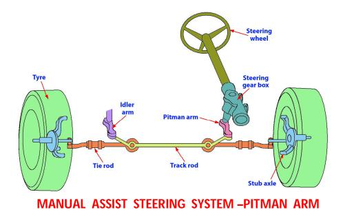
So now let us move ahead and then like look at manual assist steering systems so if we go up you know like manual assist steering systems are gear assisted right. So as we have already seen we have a rack and pinion and a worm gear based system so first let us look at worm gear based steering systems or what is generally called as pitman arm type steering? Okay so this is the one which is based on worm gears.
