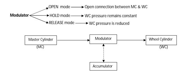
**COMPONENTS OF ABS- FLOW CHART OF OPERATION**
