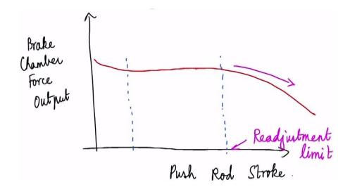
So if we plot the brake chamber force output this is push rod stroke what is going to happen is the following. We are going to see a drawing a diagram something like this for most operating pressures ok so some characteristic curve like this. So typically if you install a new brake lining we are going to have some base line stroke let say around half an inch right that is a typical stroke such that the drum brake is properly apply.
