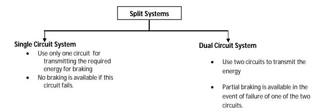
So, imagine that you know like we had only one point of control for the driver and there is only one essentially circuit you know like let it be hydraulic, mechanical or compressed air that provides this energy to let us say all the wheel; the brakes on all the wheels, right. So, use only one circuit for transmitting the energy required for braking, okay and obviously, if there is any failure in this or fault in this circuit that is going to be very detrimental, right.
