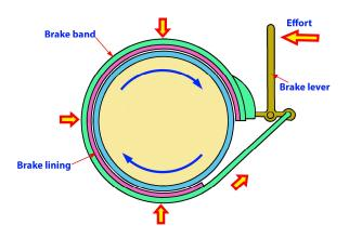
So initially what happened was that wheels were braked the initial mechanism were all mechanical were braked by wedging a shoe against the rim. So what this means is that let us say you know like we have a wheel okay. If you compare a horse driven carriage and so on right? You have a wheel and typically what happens is there is a brake shoe and that is essentially controlled by a lever which go which is under the control of the driver.
