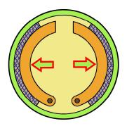
of the drum rather than the external surface. Okay so that led to what is called as an internal expanding brake. Okay what we typically see as a drum brake. So today drum brakes are used along with disc brakes as common friction brakes in road vehicles.
