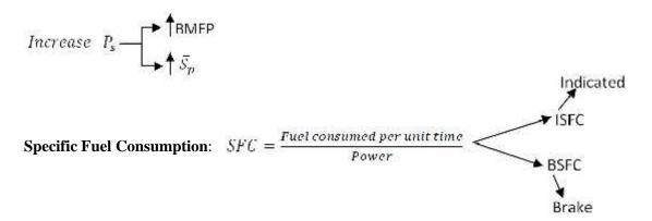
So you can immediately see that specific fuel consumption is inversely proportional to the thermal efficiency of the engine. So obviously, you know higher the thermal efficiency, lower is a specific fuel consumption and that is what is desirable to us right. Because I want to consume as less fuel as possible for delivering at given power output ok, so we want low specific fuel consumptions ideally right to the maximum possible extent.
