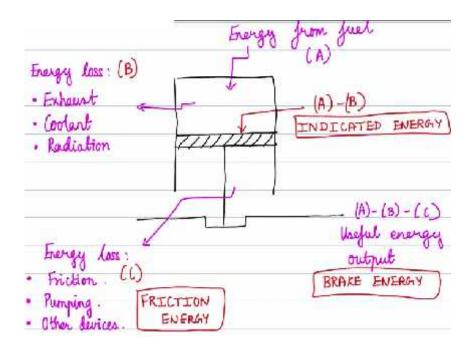
DIFFERENT ENERGY GENERATED AND LOST FROM IC ENGINE
