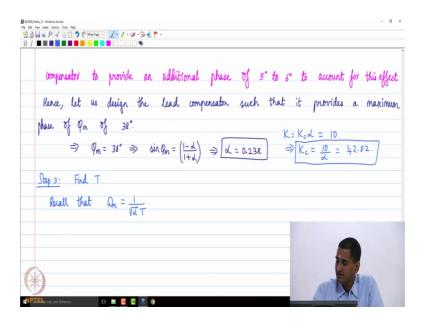
Hence, let us design the lead compensator, such that it provides a maximum phase of phi m, you member what phi m was right, phi m was the maximum phase contribution right, for the lead compensator factor.
