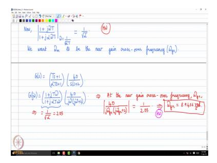
So, this expression I leave you to you as homework. The magnitude of 1 1 plus j omega T divided by 1 plus j alpha omega t at omega equals 1 divided by square root of alpha times T that is going to equal to 1 by square root of alpha ok.
