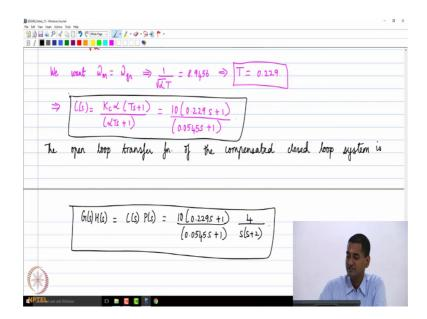
So, now, note that we want omega G n oops, we want omega m. What is omega m? Omega m is the frequency, where the lead compensator provides the maximum phase ok, to be omega G n and what is omega m? 1 divided by square root of alpha T.
