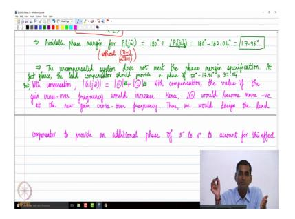
With compensation, the magnitude of G of j omega is going to be magnitude of 1 plus magnitude of 2 in decibels right. So, with compensation consequently the value of the gain cross over frequency would increase ok. Hence, the phase of 2 would become more negative at the new gain cross over frequency right.
