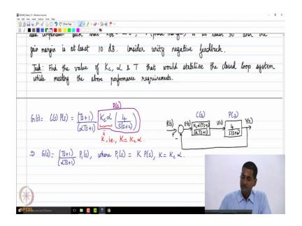
So, the plant transfer function is going to be 4 divided by S times S plus 2 right. So, this is U of s and we get a y of s out of it right.
