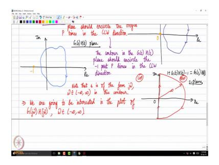
So, if you look at the s-plane, what is the contour that we are considering it is a semicircle of infinite radius that goes from minus j infinity to plus j infinity then sweeps the entire right of plane and then comes back all right. So, this is like infinite radius right LHP and RHP ok. So, this is an semicircle of infinite radius that sweeps the entire right of complex plane is it not ok.
