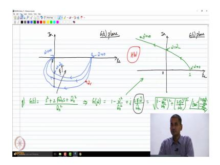
So, then you also need to do the reciprocal so that is g. What is a reciprocal it is going to be s square plus 2 zeta omega n s plus omega n square divided by omega n square. So, this implies that G of j omega is going to be 1 minus omega square by omega n square plus j times 2 zeta omega by omega n that is the real part and the imaginary part.
