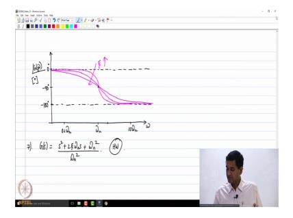
So, let me plot the phase plot of this particular transfer function. So, this we are going to plot in degrees. So, let us say this is 0 or minus 90, then minus 180, then we have omega n 10 times omega n and 0.1 times omega n, ok.
