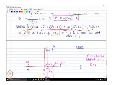
Now, we substitute s equals j omega into this particular equation right. So, this is the closed loop characteristic equation right, because please remember, the roots of this closed loop characteristic equation are the closed loop poles right. So, we are looking for closed loop poles, which are which are what to say imaginary.
