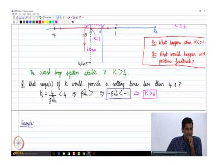
And immediately we can see from the root locus is that the closed loop system is stable for all K. When is the closed loop system stable?
