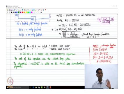
If we had a MIMO system, Y(s) will be a vector and U(s) will be a vector, then what we have is a transfer function matrix. In that case we need to be careful about the order of multiplication of two transfer functions. For example; multiplication of C(s)P(s), we cannot write it as P(s)C(s) because they are matrices.
