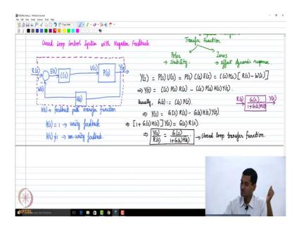
The advantage with going to the complex domain and drawing this block diagram is that the output signal at the plant block (Y(s)) right is going to be the product of the block transfer function and the input to the block.
