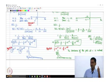
the consequence of the introduction of the zero at -2 which is closer to -1 is that the dominance of the pole at -1 is reduced. As we keep on moving the zero closer and closer to -1, the dominance of the pole at -1 will keep on reducing further and further.
