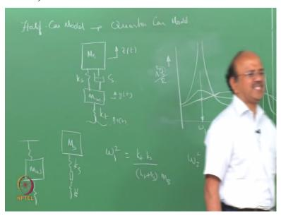
So I can actually look at it as if there is small mass here, okay as if it is going to be like that and 2 springs in series with a mass Ms so that omega 1 square is written as k/M, okay, so this is k spring, k tire, k tire\*k spring/k tire+k spring\*Ms, okay. So, this is very straightforward, in fact, you can achieve that by an approximate, say for example you can do a Taylor series approximation here and you will get a very similar result right.
