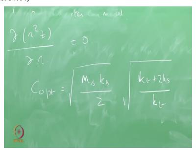
In other words, when they duo of omega 2 z, of course r is what is a given as a constant this=0 okay. This is the first cut optimized c. so the result is that c optimized = root of Ms\*ks/2\*root of kt+2ks/kt.
