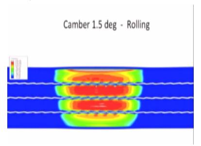
These things have an important effect on the wear of this rib tires and these factors usually make the tire not to wear uniformly, okay there would be an uneven wear in that tire, why is it so? Quickly look at; so you can see the difference between that is the contact pressure distribution when you have a camber. The camber is a very tricky business, the whole; it changes the world contact pressure distribution and hence it changes the wear.
