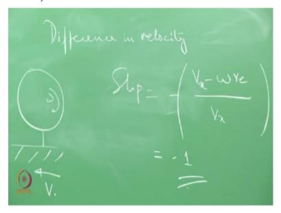
Now, we have lots more to cover, so let us go a bit faster, let us understand 3 things; the traction, braking and cornering before we derive simple formula in order to appreciate the physics that we are going to bring in here okay. One thing is very clear from what we did in the last class, on the classes before that there is a difference in velocity okay, difference in velocity, what is the difference; Velocity between the tangential velocity and the ground velocity; right.
