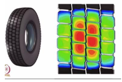
If you look at a lug tire you, would see a number of; you know lateral channels for taking or removing water, okay as it goes along. What is called as hydroplaning? Is avoided in this kind of lug tire, hydroplaning here I am using in the sense that there would be a water film that is formed and the friction coefficient reduces and so on, which will see again in the next couple of classes okay, so there are channels for the water to be carried.
