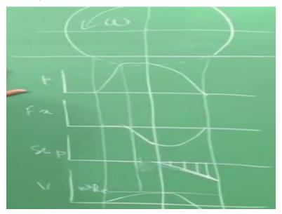
Sir, what is the actual thing if the wheel is moving? Here, the wheel is rotating, okay so, omega is present but there is no grip, so the vehicle is not moving, you would have seen this many times, you know if in water, the wheel rotates, the vehicle is not moving or in sand, it does not
