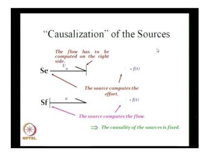
So, here is the explanation for causalization of the sources. So, now, we have this s e and SF s e is the source efforts and SF is the source flow. So, the flow has to be computed on
