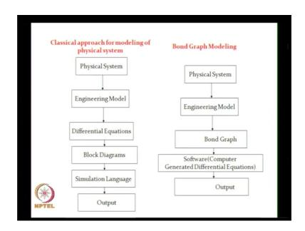
And this diagram, I explained the difference between the normal or conventional way of modeling and the bond graph modeling. So, here basically we do not go for the differential equations instead we directly go for the bond graph models or direct from the physical system, we develop a an engineering model of system and then convert that in to a bond graph and then we can use the standards software for simulation. So, that is the main difference in bond graph and the classical approach.
