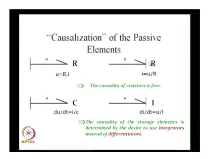
And for other elements to fix the causality for the other elements we need to actually find out the relationship for these elements. So, here you can see this is the R element and for R element we can actually have a relationship like u is equal to R multiplied by I or I is equal to u divided by R that is how you calculate the.
