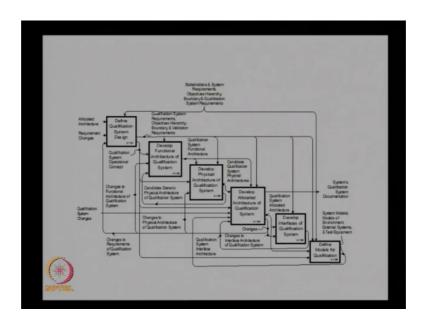
So, if you look at the IDEF 0 diagram for the same process you can see that these are the inputs going to the system that allocate the architecture requirement changes then we have or their inputs and there is functions we have 1, 2, 3, 4, 5, 6 functions in the qualification system design and finally you will be getting the system qualification documentation I will show you a better picture over here. So, you can see here.
