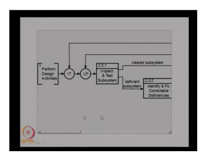
We will discuss about the function block diagram in one of the coming lectures. So, this basically the same flow chart whatever we a shown is shown as here as a function flow block diagram it represent the iterations and LP is a loop. So, we perform the design activities and then inspect and test the subsystem and the deficient subsystem will go through one channel.
