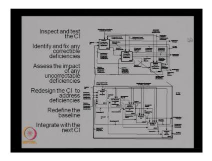
This can actually be represented by a diagram these are the stages basically inspect and test the CI identify and fix any correctable deficiencies, assess the impact of any uncorrectable deficiencies, redesign the CI to address efficiencies and redefine the base line. So, these are the stages involved and with integrate with the next CI. So, this can actually be shown as an id of zero diagram.
