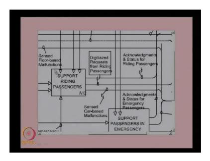
So, the input from one function will be, output from one function will be an input to another function and similarly the output will be can be one function can be input to a previous function also. So, you can divide the main A1 function into A11, A12 and A13 in this diagram. So, this diagram is basically, the A1 diagram where the A1, A2, A11, A12 and A13 functions are decomposed and their interactions are clearly as shown. So, that is the A1 diagram.
