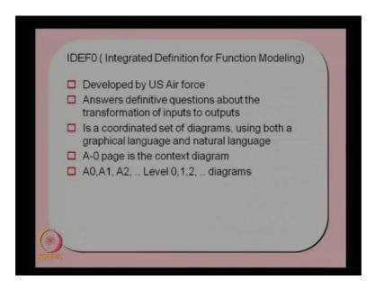
Basically, this method known as Integrated Definition for Function Modelling or in short IDEF0, 0 was added I mean is a first initial chart that is why it is known as IDEF0, it is a integrated definition for function modelling. This was developed by US Air Force in
