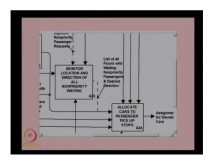
That is this is the one of the input that is allocated cars to passenger that information will be there and that information will be going to this one to monitor the location of the car. So, based on these information it will continuously monitor location of all cars and give this as an output to the other function of allocating the functions. So, and any sensed malfunction also will be given as an output.
