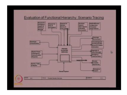
So, as I mentioned earlier, from the context diagram we can actually take any one of these inputs and you see what is the output coming from there and then we can find out what is happening to these input, as if the input goes through different functions. So, this is known as the scenario tracing. In this case, we take the request for elevator service and entry support as an input and see the output as elevator entry exit opportunity. So, customer is giving, different diagram.
