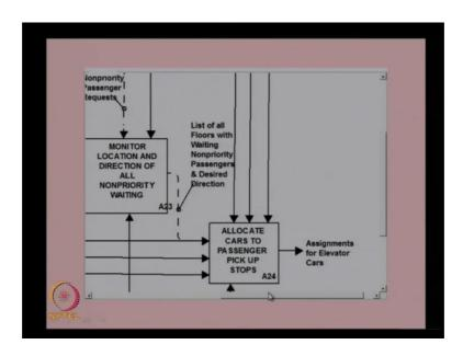
So, we can see here the control elevator cars is a function in order to satisfy the requirement in has to provide the sub functions like monitory location of all cars then monitor location and direction of all priority passengers as well as the monitor location of non priority passengers and this information will be used by the function to allocate cars to different floors. So, that is the decomposition of A2 function in to A21, A22, A23 and A24.
