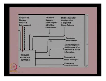
Similarly, the structural support, alarm signals and building environment and modified elevator configuration and expected usage patterns. This is basically from the patterns that also will be given as an input to the system. So, these are all the inputs going to the system and the output coming from the system are the passenger environment, what is
