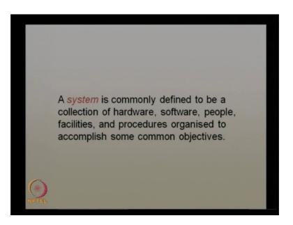
So, like this there are multiple definitions, standard definition is basically a system is commonly defined to be a collection of hardware, software, people, facilities, and procedure organized to accomplish some common objectives. So, that is a common definition for engineering system which is a collection of hardware software people and other facilities in order to get to accomplish common objectives.
