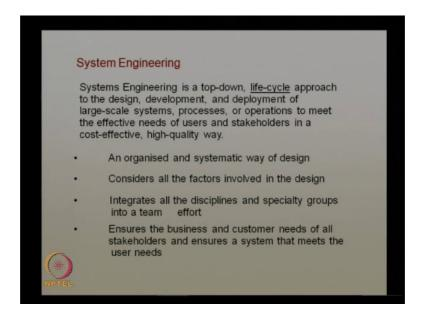
So, let us see the what are the important points we need to discuss or we need to learn when we design this kind of a complex engineering systems, to define the system engineering basically it is a top down lifecycle approach to the design, development, and deployment of large scale systems, processes, or operations to meet the effective needs of users and stakeholders in a cost effective high quality way.
