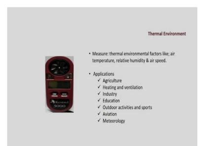
Now, this is a very interesting instrument. This is apart from that we have many other we call a "thermal environment meter". So, let us talk about the thermal environment. So, this is one instrument which measures air temperature, relative humidity, and air-speed. We have some instrument which can measure you know air temperature separately, dry and wet.
