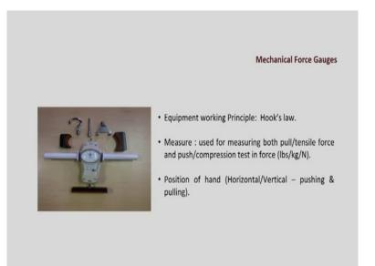
Now, another very important instrument that we normally use is the mechanical force gauges. This particular instrument is being used for pull or push that is the major use of this particular instrument, and the reading is being recorded by the pound, kg, or Newton. This instrument is based on "Hook's law". So, now I am not going to tell in detail of all these instruments. So, if you find this particular instrument is useful or this particular variable is useful for your
