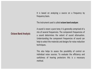
In octave band analysis it is basically is analysing a source on a frequency by frequency basis. So, the instrument used for this particular method or process we call it as octave band analyser.
