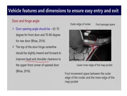
So, as we discussed earlier, the outer edge of the rocker panel and the lower inner edge of the door panel. So, this gap, this angle is very crucial for the entry/exit process because through this area actually; leg, feet come out or goes in. So, for this purpose, foot movement space between the outer edge of the rocker and the inner edge of the map pocket should be sufficient enough.
