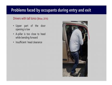
So, they find that the upper edge of this roof rail is low, the height of the roof rail is relatively low for them; they need to bend-forward. First, they hold the steering wheel; then they need to go inside. So, this dimension is not appropriate for them.
