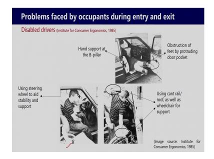
In this report by the Institute for Consumer Ergonomics (1985), it was also reported; various problem faced by the disabled drivers. So, as it is shown, in this image, the person is using a steering wheel to aid stability and support. Here, it is shown that he is using cant rail or roof as well as the wheelchair for the support while going inside or coming out.
