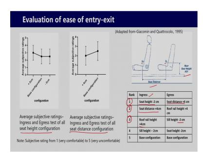
So, they asked the subjects to rate the rating scale, where 1 is very comfortable, and 5 is very uncomfortable, for different vehicle components. So, for a sill height, so, average
