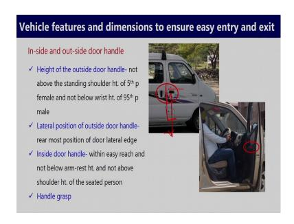
Now, inside and outside door handle. So, from this image, you can see, these are the outside door handles, for the front compartment, that is for the driver compartment, and this is the backside compartment, for the passengers. So, how should be the design of this door handle, and how should be the dimension? So, if we consider the height of the door handle from the ground. So, if we decide the height from the ground, then how much that height should be?
