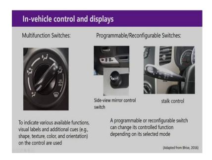
There are also multifunctional switches, here is one example. So, this is for the control of the AC vent, the direction of the airflow, whether it will come from the front and towards the leg. So, different types, if we rotate this control, then we can set it at different positions and accordingly we will be able to achieve different types of settings.
