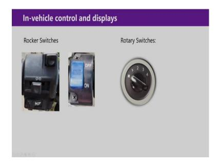
Now, there are also other types of controls like rocker switches, different types of switch for on and off. So, if we press one side, then another side will be protruded, and when we press another side, then the opposite side will be protruded. So, based on that, we can understand whether that is in on and off opposition; otherwise we can move different types of rocker switches; left to right. Also, this type of button switches for horn. So, these are the examples of rocker switches.
