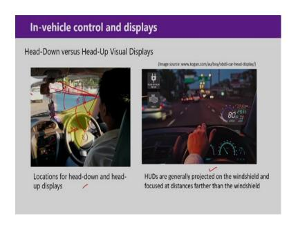
So, first, we should know what is head-down display? And what is the head-up display? So, if you look at this image, then, while driver is looking straight forward; below that straight-forward line of sight, if you go up to 35-degree down. Generally, it is starting from 15-degree; this is for outside visibility.
