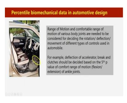
Now, apart from the anthropometric data, biomechanical data is also important for automotive component design. For various component operations, either that is foot control or different types of controls on the dashboard, it requires a different type of range of motion of our hand or leg, at the same time different amount of force is required for actuating those controls.
