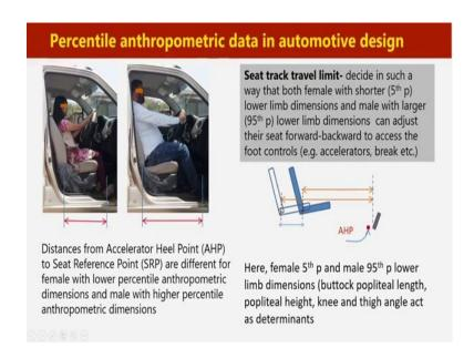
Now, if we think about the seat track travel limit. So, how much should be the seat track travel limit? So, for that purpose, if we look at this image; for female with shorter body dimension, they adjust the seat forward, so that they can access the foot controls, at the same time they can hold the steering wheel. On the other hand, male with larger body dimension, they move the seat backwards, so that they can sit comfortably, access the steering wheel and foot controls.
