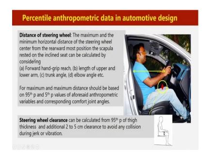
Now, the distance of steering wheel; the steering wheel centre to the seat back distance. So, the maximum and minimum horizontal distance of the steering wheel centre from the rearmost position of the scapula rested on the inclined seat can be calculated by considering these variables; one is forward hand-grip reach, length of upper and lower arm, trunk angle and elbow angle. So, based on these variables, we can calculate how much these maximum and minimum distance should be there.
