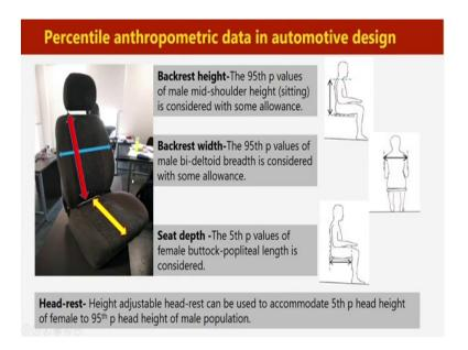
Now, for backrest height, this dimension. For backrest height; which is the corresponding anthropometric variable? For this purpose, anthropometric variable which we should consider that is the mid-shoulder height.
