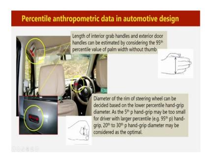
Now, various other vehicle components which are also needed to be designed based on the anthropometric variables. For example, when we are positioning this type of interior grab handles or door handles, then we need to consider this hand dimension and that hand dimension is the 95<sup>th</sup> percentile palm width.
