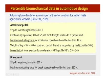
Generally, while we are deciding the actuating force, generally, lower percentile, means, 5<sup>th</sup> percentile force value of leg strength or hand strength value is considered. So, that the majority of the population, almost 95 percent of the population can operate that particular control. So here, from that above aforesaid reference, we are discussing some of the control operations and its corresponding actuating force requirement. So, this is mainly for tractor design.
