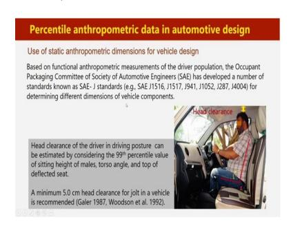
See, first; use of static anthropometric dimension for vehicle design. So, based on functional anthropometric measurements of the driver population, the Occupant Packaging Committee of Society of Automotive Engineers, that is SAE has developed the number of standards which are known SAE J standards like SAE J1516, J1517, J941, J1052, J287 and J4004. So, these various 'J' standards are there for determining different dimensions in vehicle components.
