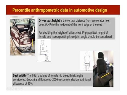
Now, driver seat height; how much should be the height of the middle of the front edge from the floor. Driver seat height is the vertical distance from the Accelerator Heel Point (AHP) to the mid-point of the front edge of the seat. For deciding the height of this driver seat, 5<sup>th</sup> percentile popliteal height of female and corresponding knee joint angle should be considered.
