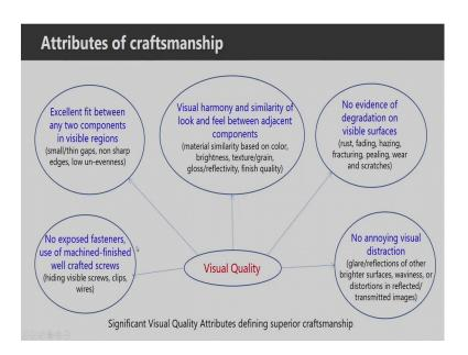
We will discuss individually about these various factors and how visual quality is associated with superior craftsmanship. There should not be exposed fasteners and there should be use of machine-finished well-crafted screws. To achieve these things, what we need to do? For hiding visible screws, they should be covered properly, there should not be any clips wires visible from the outside. There should be excellent fit between any two components invisible regions.
