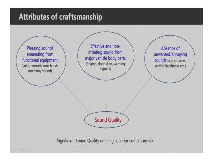
Another important aspect associated with the craftsmanship is the sound quality. What type of sound that the user will perceive while they are operating that vehicle either opening or closing or going inside? The pleasing sound should be solid, and smooth. The sound should not be harsh or tinny sound. Effective and non-irritating sound from major vehicle body parts like engine, door slam, warning signals.
