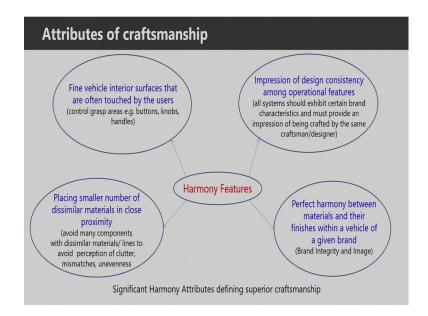
The next important aspect is harmony features. So, how the designers can maintain the overall harmony among various components and sub-components of the vehicle? For that purpose, placing small number of dissimilar materials in close proximity should be avoided. Avoid many components with dissimilar materials, lines to avoid perception of clatter mismatches and unevenness.
