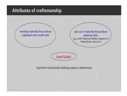
Also, the smell quality is directly associated with the perception of the craftsmanship of the automotive product. We have to try to avoid materials that produce unpleasant and unsafe odor. Because while the drivers or any user or customer going to buy a new car or looking at the car there should not be any an unpleasant smell from that vehicle. On the other hand the smell coming out from the vehicle or vehicle component it should be very pleasant.
