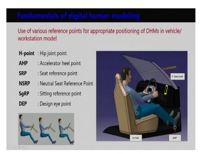
After using these anthropometric and biomechanical database, when you are developing the digital human models of varying percentile as per your requirement, now the question is coming how you will position those digital human models inside the vehicle or any other workstation. So, for that purpose for proper giving appropriate posture and positioning the digital human model inside the vehicle or cab model or any other workstation model we need some reference points.
