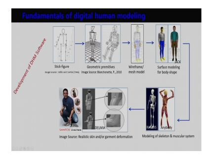
If we look at this particular slide, we can see that how gradually digital human modeling software evolved. It started from the stick figure like appearance gradually to move to geometric primitives like overt like appearance, then wireframe like model, shaded model with surface modeling with smoothing algorithm we can see this type of dressed model.
