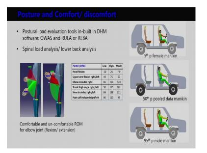
How we can use digital human modeling software for evaluation of posture and comfort discomfort? As we discussed earlier for comfort discomfort evaluation it is important to understand the range of body motion, a range of body joint/ ROM and at the same time the comfort range of motion within the total range of body joint movement.
