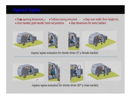
Apart from this, vision analysis digital human modeling software is also helping in ingress-egress analysis. So, various aspect of ingress-egress analysis meanwhile the driver or passenger is going inside the car or any other automotive vehicle and coming out then what type of problem they are facing and how much is or how much comfortable that entry-exit we can evaluate using digital human models.
