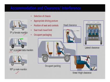
So, how we use digital human modeling software for the evaluation of various types of vehicles? First, we start with the selection of chassis. So, we think about the chassis model in the CAD software, and what will be the size and dimension? Then after the chassis is finalized, we give the appropriate driving posture of the drivers or other
