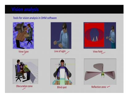
For example, there is this type of view cone where we can create view cone of varying angles. It is shown that we can create view cone of 15 degree, 30 degree as per our
