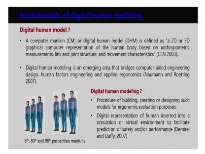
Now, what is digital human modeling software, and what is the digital human model? First, the digital human model is a computer-aided manikin or digital model which is defined as the two dimensional or three-dimensional computer graphics representation of human body; based on anthropometric and biomedical data measurements link and joint structure movement characteristics as defined by CEN 2003.
