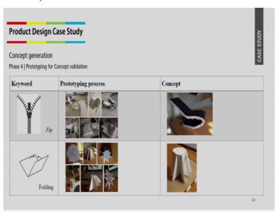
Using those actions, we have started making our prototypes for concept validation for example, using this zip action where two sides are coming and joining, using that action we have started making prototypes, using that what are the kind of furniture we can use where initially it will be a sheet and whenever required we will be joining them and it will take this particular shape.
