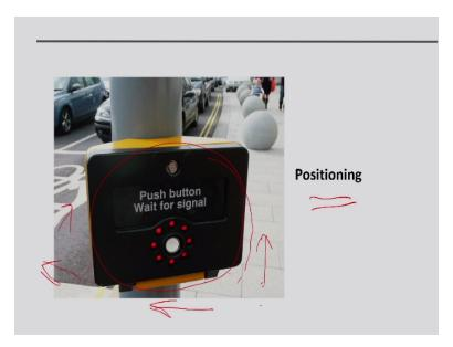
This is one example of positioning of any product; it is a pedestrian traffic signal. If you are seeing this product has been this is the footpath and this is the road. So they have put this signal in a right hand side of the person, as the person might cross from this foot path and use this road to cross. So once we will cross this road then it will be obviously we are seeing the right hand side of the road.
