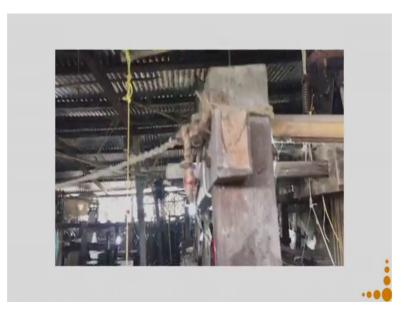
You can here see how the whole loom works. So, this is the thread connected to the jacquard and then it is connected to his peddles, which are operated by his legs.
