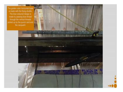
So, this one happens automatically because it put over here in the slot, and when the weaver pulls this thread, this shuttle makes travel from this point to this point. Then again the weaver will pull this shuttle will travel from this point to this point now comes how to make this designs.
